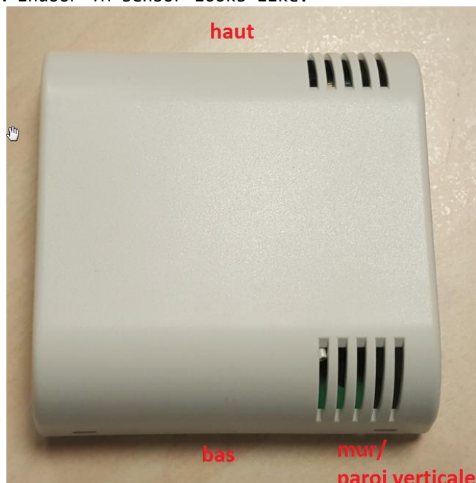
Picture 1 Sensor fixed on a vertical wall
