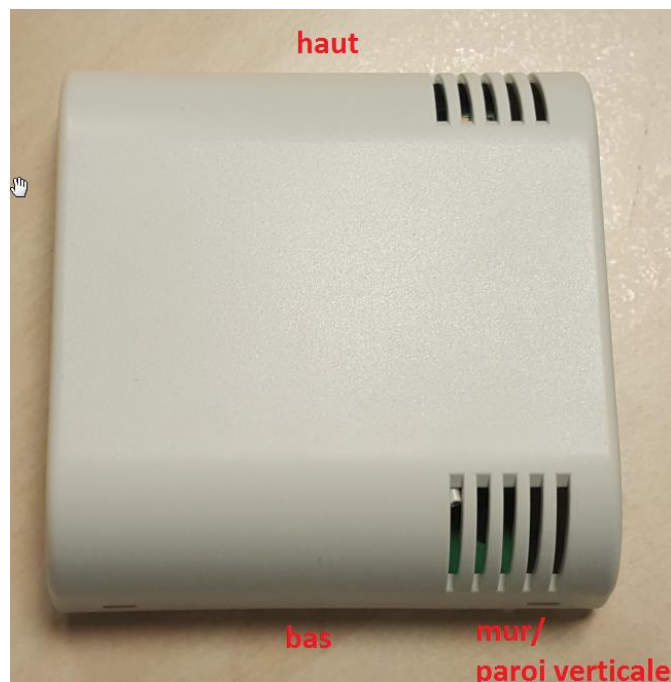
Picture 1 Sensor fixed on a vertical wall
