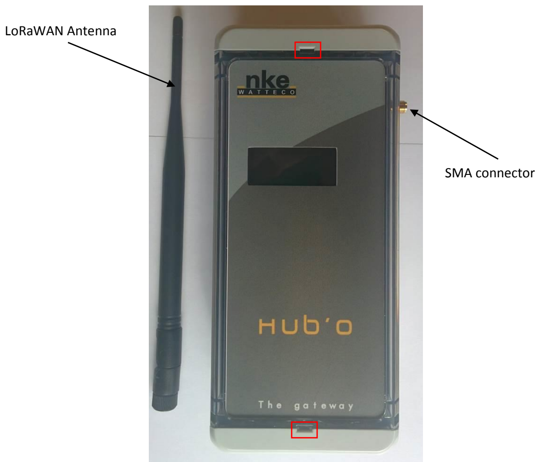
FIGURE 2 - LORAWAN GATEWAY AT RECEPTION
