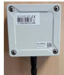
**Important:** to get the best radio coverage, the box should be fixed to the support in such a way that the stickers are can be read normally/horizontally.
